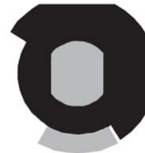
Correct stop cam placement in closed position
